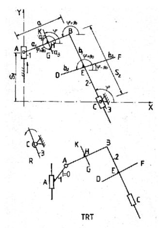
Fig.1. The kinematic scheme of the mechanism
